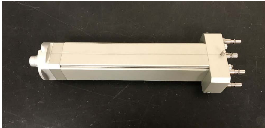
Figure 1: MURR GE ® standard cyclotron radioisotope production target.
